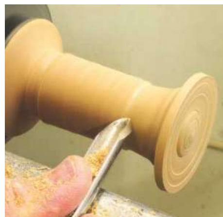
▲ Pic.18 Remove as much of the waste as you can while it's being held in the chuck. Les has reduced it to about 25mm in diameter but you could take it down even more
